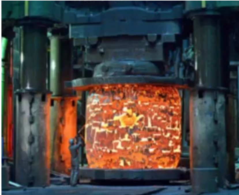
Forging steps at RDN: Up setting.
