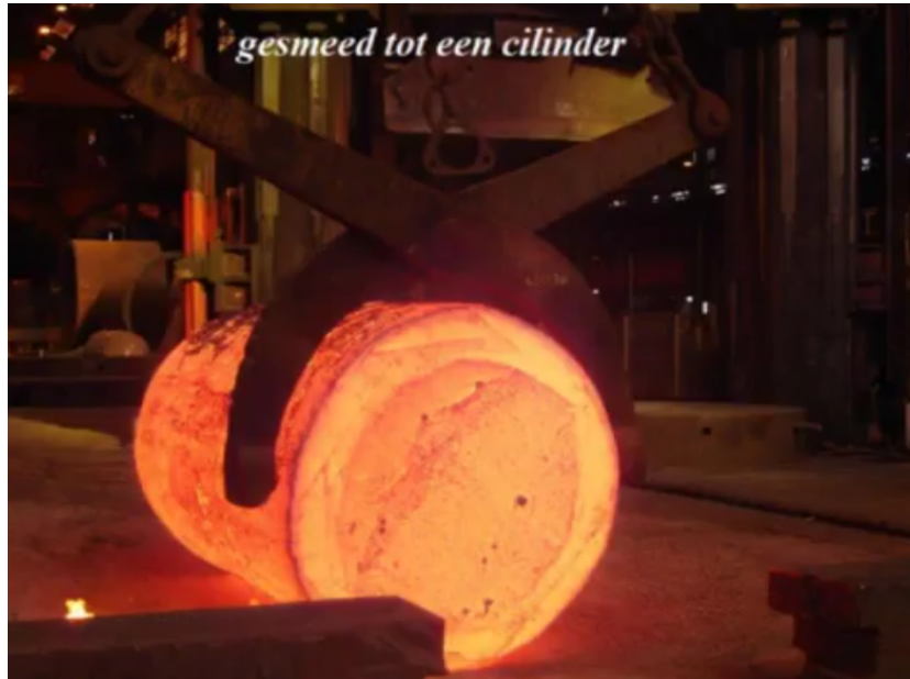
Preforging to bloom 110 ton.
