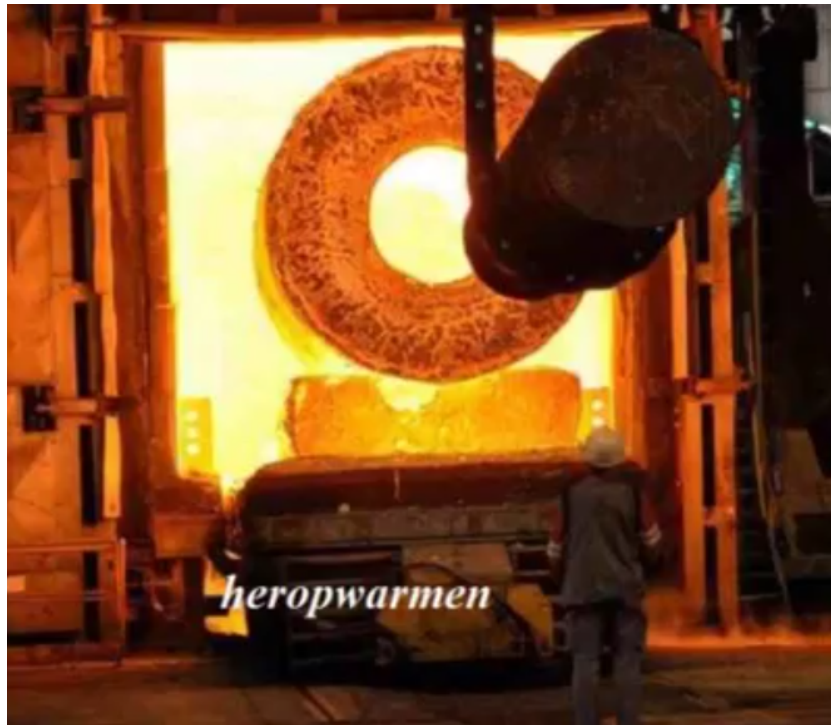
Forging steps at RDN: Pierced cylinder.
